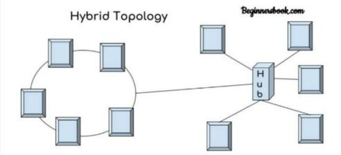
A combination of two or more topology is known as hybrid topology. For example a combination of star and mesh topology is known as hybrid topology.
