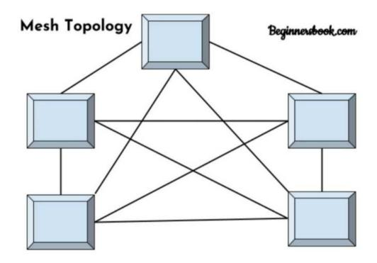
In mesh topology each device is connected to every other device on the network through a dedicated point-to-point link. When we say dedicated it means that the link only carries data for the two connected devices only. Lets say we have n devices in the network then each device must be connected with (n-1) devices of the network. Number of links in a mesh topology of n devices would be n(n-1)/2.
