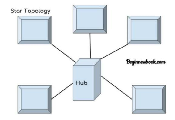
In star topology each device in the network is connected to a central device called hub. Unlike Mesh topology, star topology doesn't allow direct communication between devices, a device must have to communicate through hub. If one device wants to send data to other device, it has to first send the data to hub and then the hub transmit that data to the designated device.
