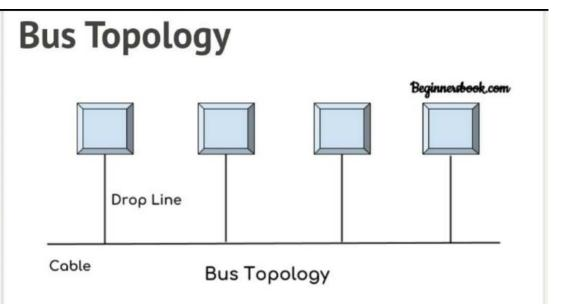
In bus topology there is a main cable and all the devices are connected to this main cable through drop lines. There is a device called tap that connects the drop line to the main cable. Since all the data is transmitted over the main cable, there is a limit of drop lines and the distance a main cable can have.
